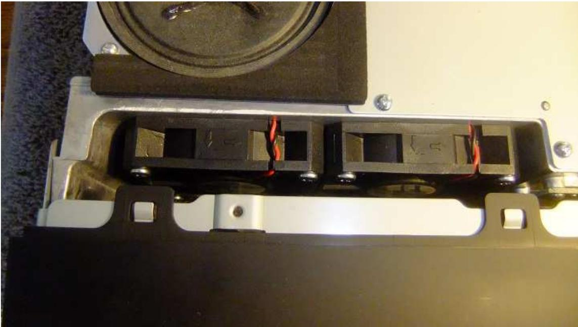
Loosen the bottom screws and remove the top screws at the sides of the front panel. Do not remove the bottom screws.
