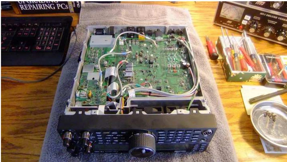
Turn the radio over, remove four more screws and lift off the top case:
