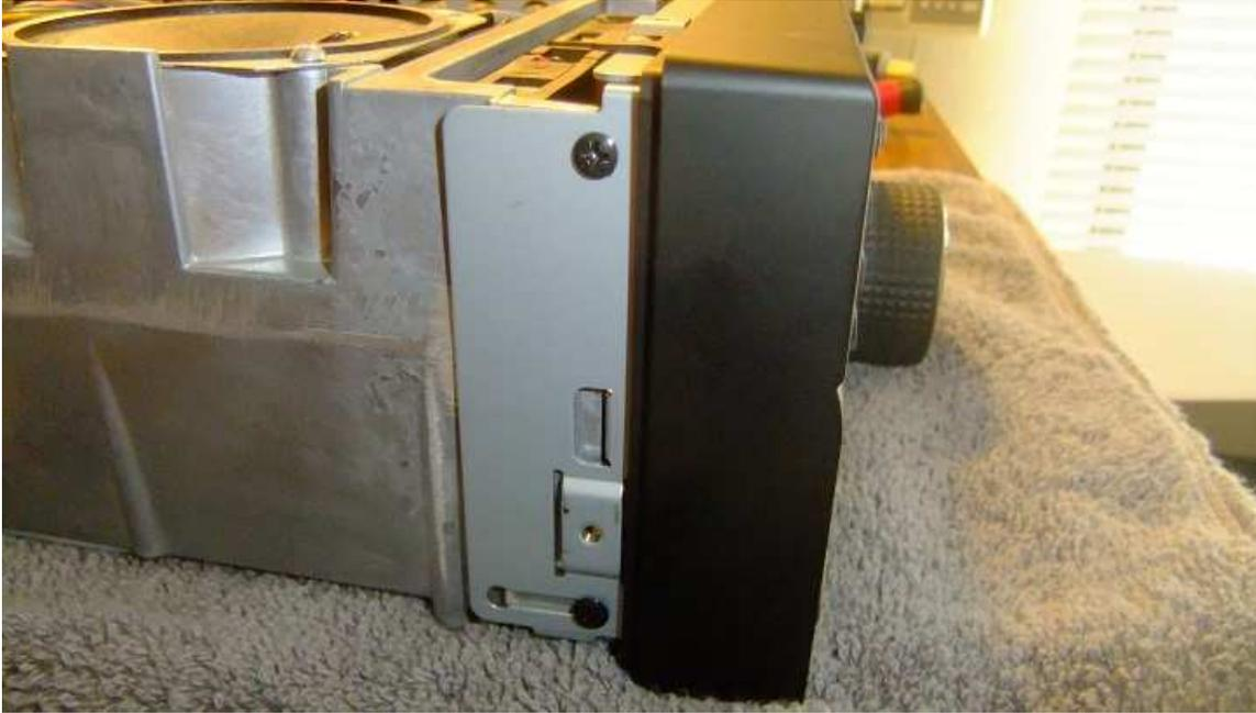
Allow the front panel to tilt down out of the way over the edge of table or workbench. You do not need to disconnect any wires. I removed the sheet metal shield on the top of the chassis, but found that was not necessary.
