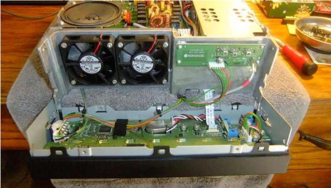
Remove the fan mounting screws and carefully lift the wires out of the notches in the fan frames. Turn the fans around and reinstall them with the air flow arrows pointing toward the back of the radio.
