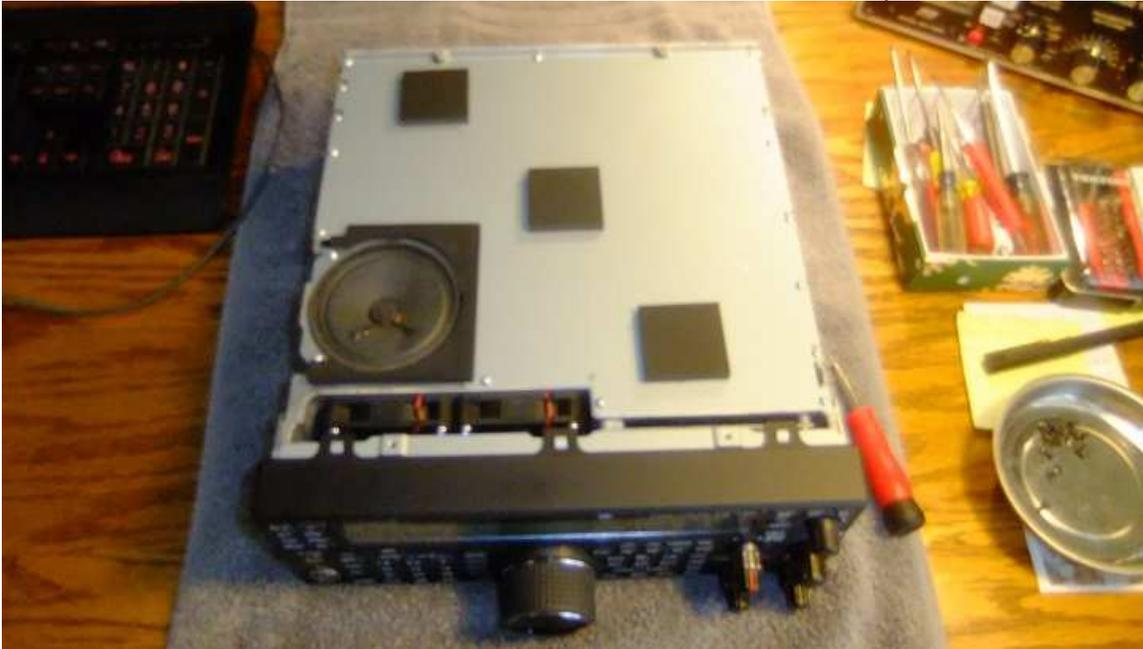
Arrows embossed on these two cooling fans show air flow is incorrectly directed toward the front of the radio:
