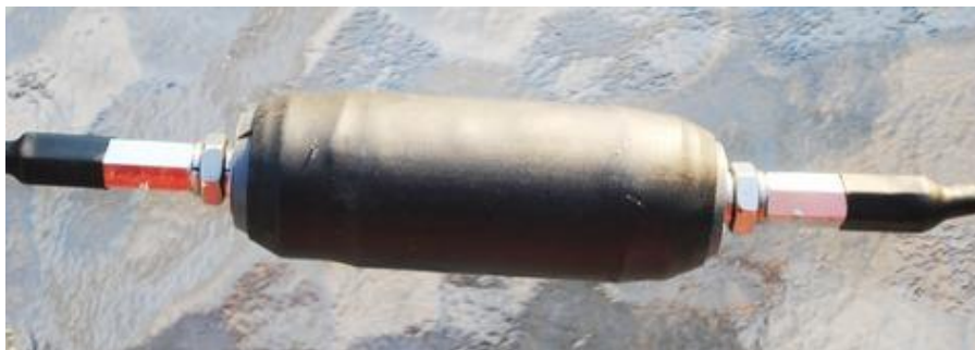
Figure 2a - Coil (or Choke) for 40m operation
